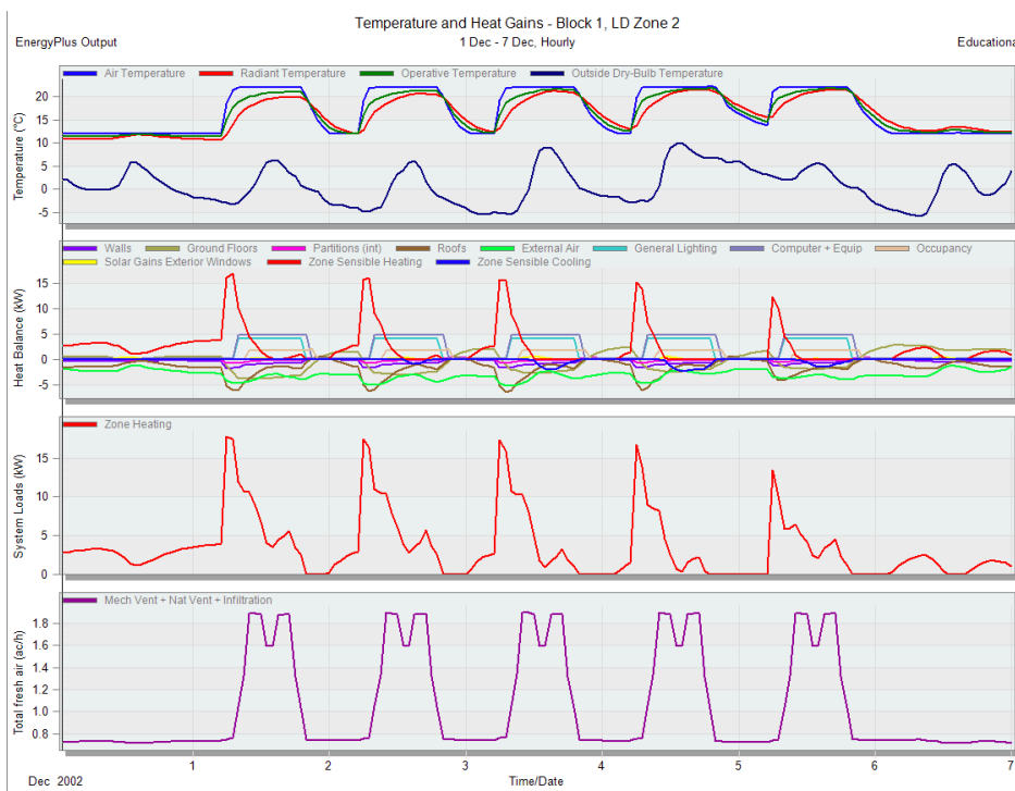
Figure 20. Graph showing Temperature and Heat Gains of Zone 2 during Winter Design Week
