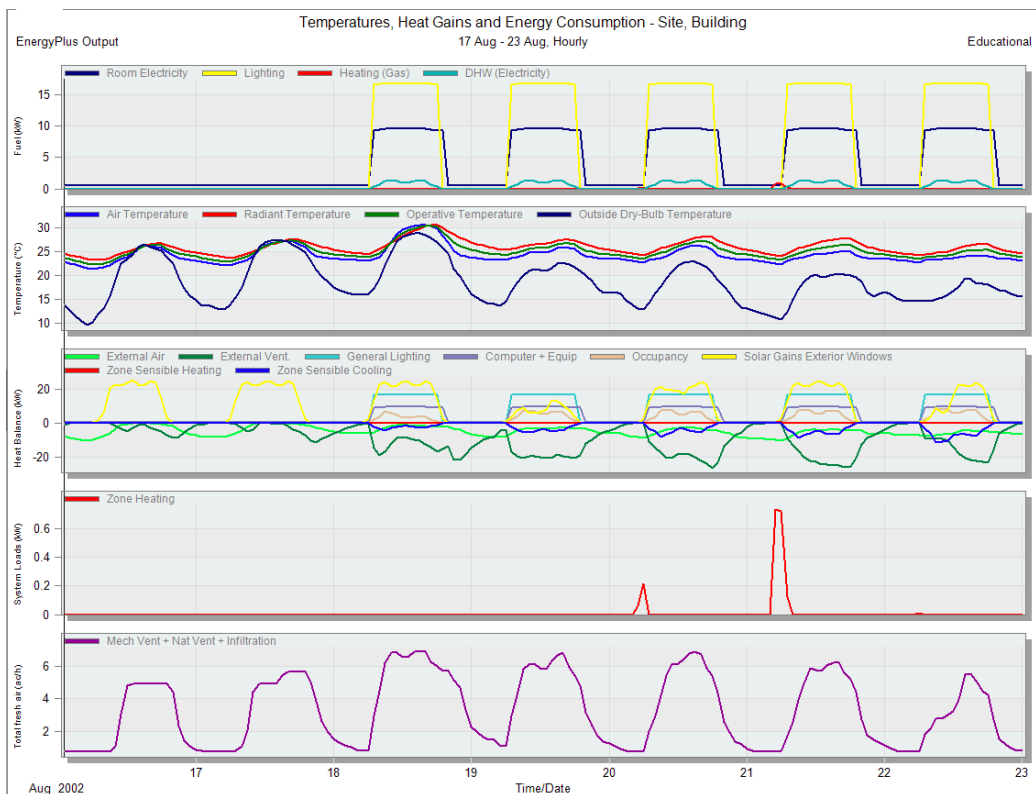
Figure 37. Graphical Representation of Temperatures, Heat Gains and Energy Consumption for the Building after defining the Ventilation Setpoint Temperature
