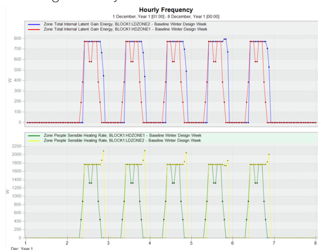
Figure 14. Graph comparing Internal Heat Gains of Zone 1 and 2 during Winter Design week
