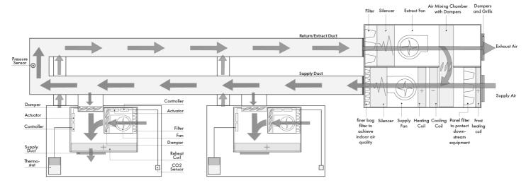
Figure 1 Basic HVAC system with VAV
